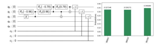
Figure 2. The quantum circuit for 3-qubit W quantum entanglement state and its probability distribution [11].
