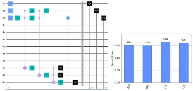
Figure 6. The quantum circuit implementation corresponding to the rule of  $n_2$  and the probability distribution of quantum entanglement states after  $n_2$  has been privileged and made a move.
