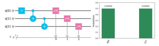
Figure 1. The quantum circuit for 3-qubit GHZ quantum entanglement state and its probability distribution [11].
