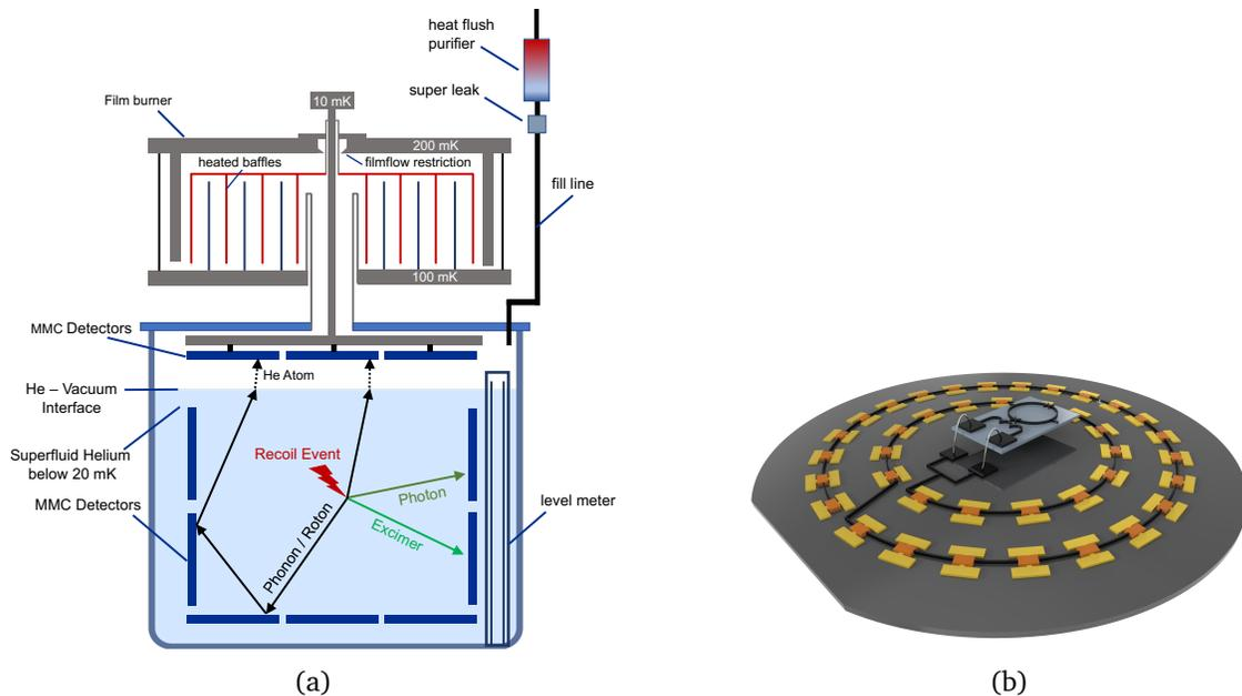
Figure 1: **a)** Conceptual draft of a DELight helium cell with film burner, heat flush purifier, level sensor and magnetic micro-calorimeter (MMC) sub-detector system. Also illustrated are the main signal channels. **b)** Schematic of a large-area MMC based sub-detector with dielectric wafer as absorber (gray), phonon collectors (yellow), paramagnetic temperature sensor (orange) and superconducting pickup coil (black) connected to a separately mounted readout SQUID [19].
