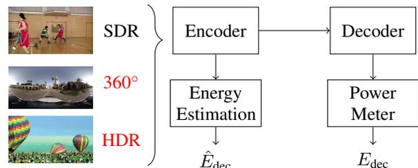
Fig. 1. Overview of the complete evaluation toolchain with the newly evaluated video formats (360°, HDR, and fisheye). First, the input sequences are encoded. Then, the decoding energy  $E_{dec}$  is measured with the help of a power meter. Energy estimation returns the modeled energy  $\hat{E}_{dec}$ , which shall approximate the measured energy  $E_{dec}$ .
