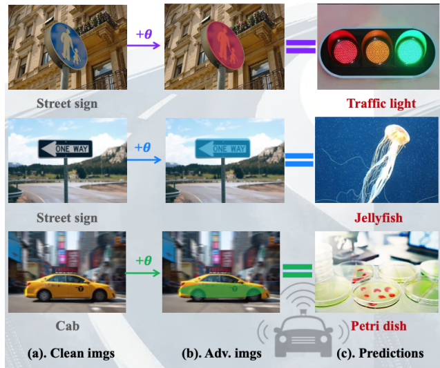
Figure 1. An example. When a camera installed in a self-driving car captures target objects that have been subjected to a carefully designed color projection attack, the object recognition system may fail to correctly identify the sign as a "Street sign" or the other objects, such as "Cab".
