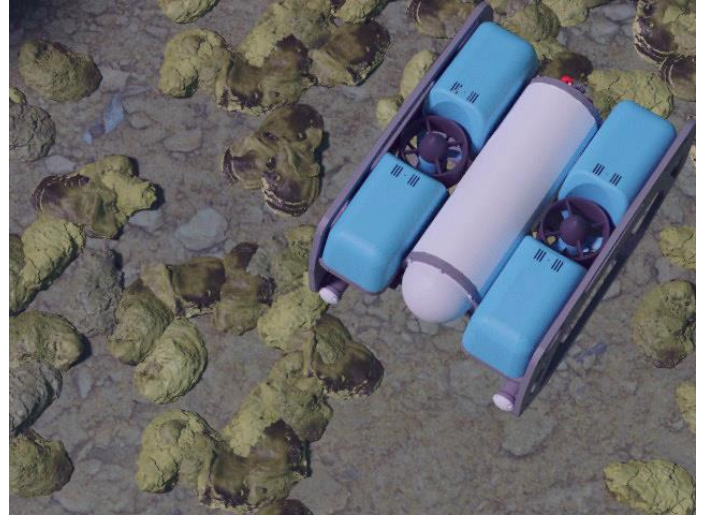
Fig. 1. Top-down view of a BlueROV navigating over an oyster reef in OysterSim environment.
