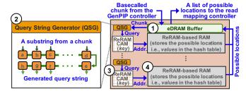
Figure 9: Microarchitecture of the in-memory seeding accelerator.
