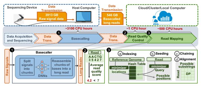
Figure 1: The genome sequencing and analysis pipeline. The basecalling step (①) and the read mapping step (②) are the two most time-consuming steps in the genome analysis pipeline. The read quality control step (②) is a highly-recommended but optional step to reduce the workload of read mapping by eliminating unnecessary computation. Dataset sizes and processing times are from [85].
