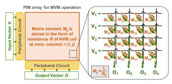
Figure 2: The basic structure of an NVM-based PIM array designed for computing an MVM operation.
