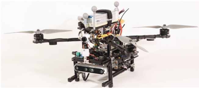
Fig. 4: The robot used in the field experiments is equipped with a forward-facing Intel Realsense D455, downward-facing mvBluefox global shutter color camera, and Pixracer flight controller.
