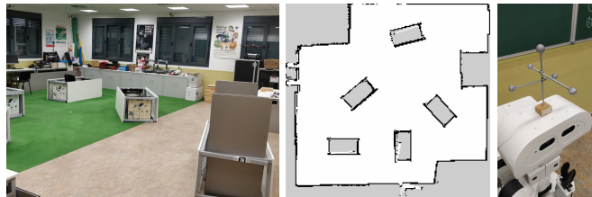
Fig. 4: Real scenario (left) and its map (center) for the first two experiments, and the motion capture object for tracking the robot (right).
