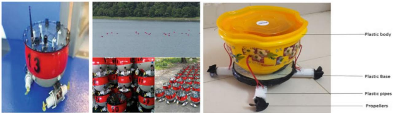
Fig. 14. Swarm of Buoys developed in Bouffanais's Lab and Waterbot
