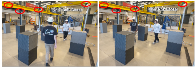
Fig. 6. Illustration of using the OptiTrack motion capture system to estimate the error of the proposed dynamic obstacle detection and tracking method.
