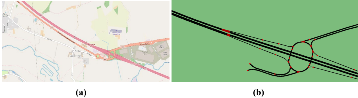
Figure 5 Southbound road segment leading to M1 Junction 16 from (a) Open Street Map and (b) SUMO
