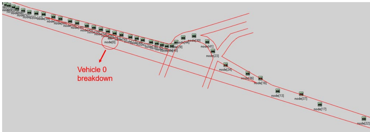
(b) Vehicle 0 breakdown in Experiment 3: CVs diverted to the alternative route once they received the warning messages
