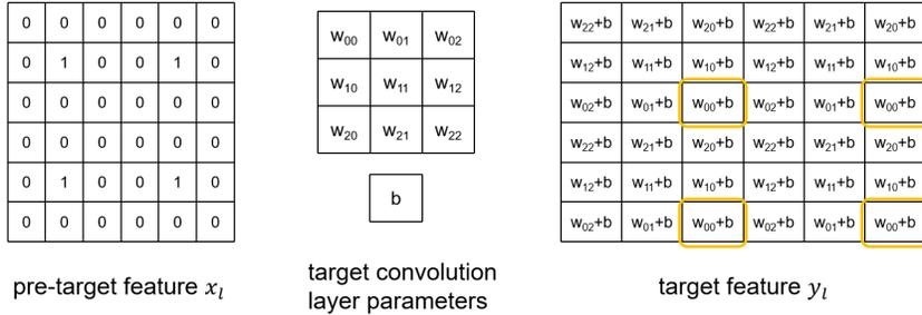
Figure 2: An example of the convolution layer extraction method, as shown in algorithm 3. For simplicity, only one channel for each layer is shown. By setting the pre-target feature  $x_l$  to be nonzero with a period of kernel size, the target feature layer  $y_l$  is also periodic, and the values in the orange boxes can be extracted together for better accuracy, which reveal the values of target convolution layer parameters.
