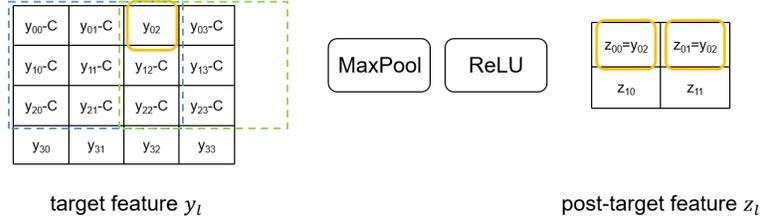
Figure 1: An example of extraction method for a maxpool-ReLU layer input feature. Features in the orange boxes are the target feature  $y_{\ell,i}$  and its related features  $Z_{\ell,i}$  in the post-target layer, respectively. The dashed rectangles are ranges of maxpool kernels.  $C$  is a large positive constant, added in order to suppress the effect from other features on  $y_{\ell}$  to  $Z_{\ell,i}$ .
