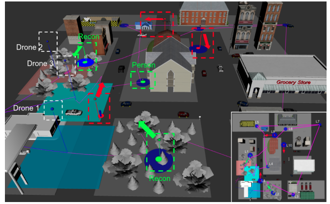
Fig. 5. Graphical depiction the environment considered in Section IV-E. The colored squares represent the field of view of our drones. Target (recon drones) movement is shown with green arrows and security drone movement is shown with red arrows.
