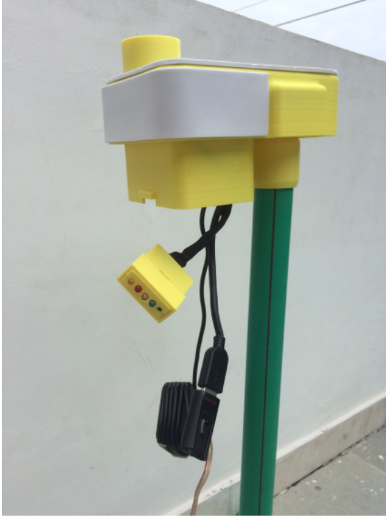
Figure 12: GSI with lid retainer and the lid removed
