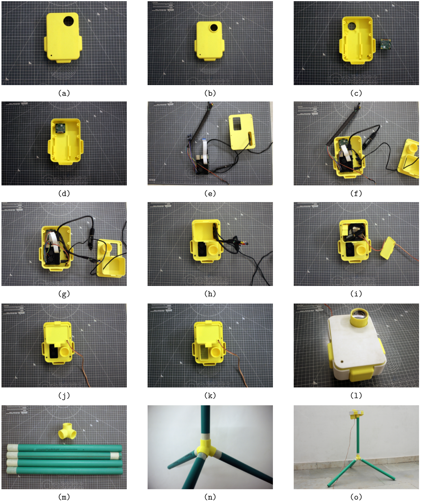
Figure 10: Assembly steps for the GSI
