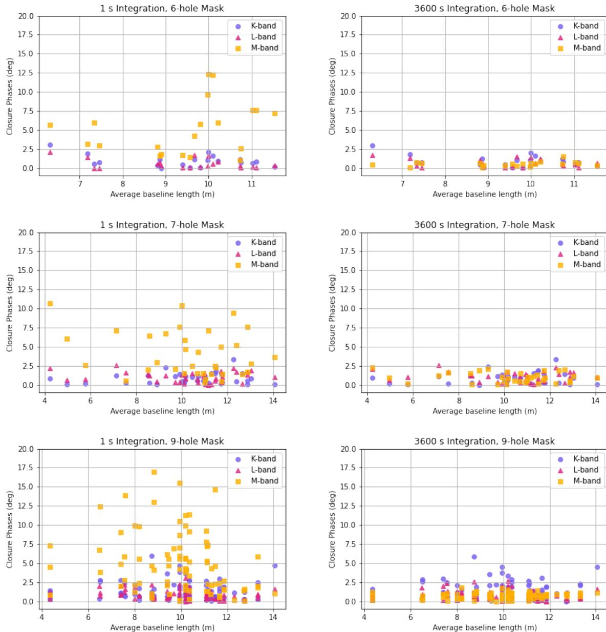
Figure 3. Absolute values of closure phases for each mask at integration times of 1s and 3600s, plotted against the average baseline length calculated for each closure triangle. Data points are shown for individual wavelength bins in the K, L, and M bands.
