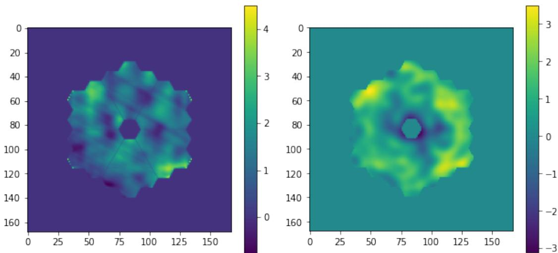
Figure 2. OPD maps used in this work. Left: average of 1 second of data sampled at 1kHz. Right: averaged OPD map evolved using a 500 degree Zernike polynomial.
