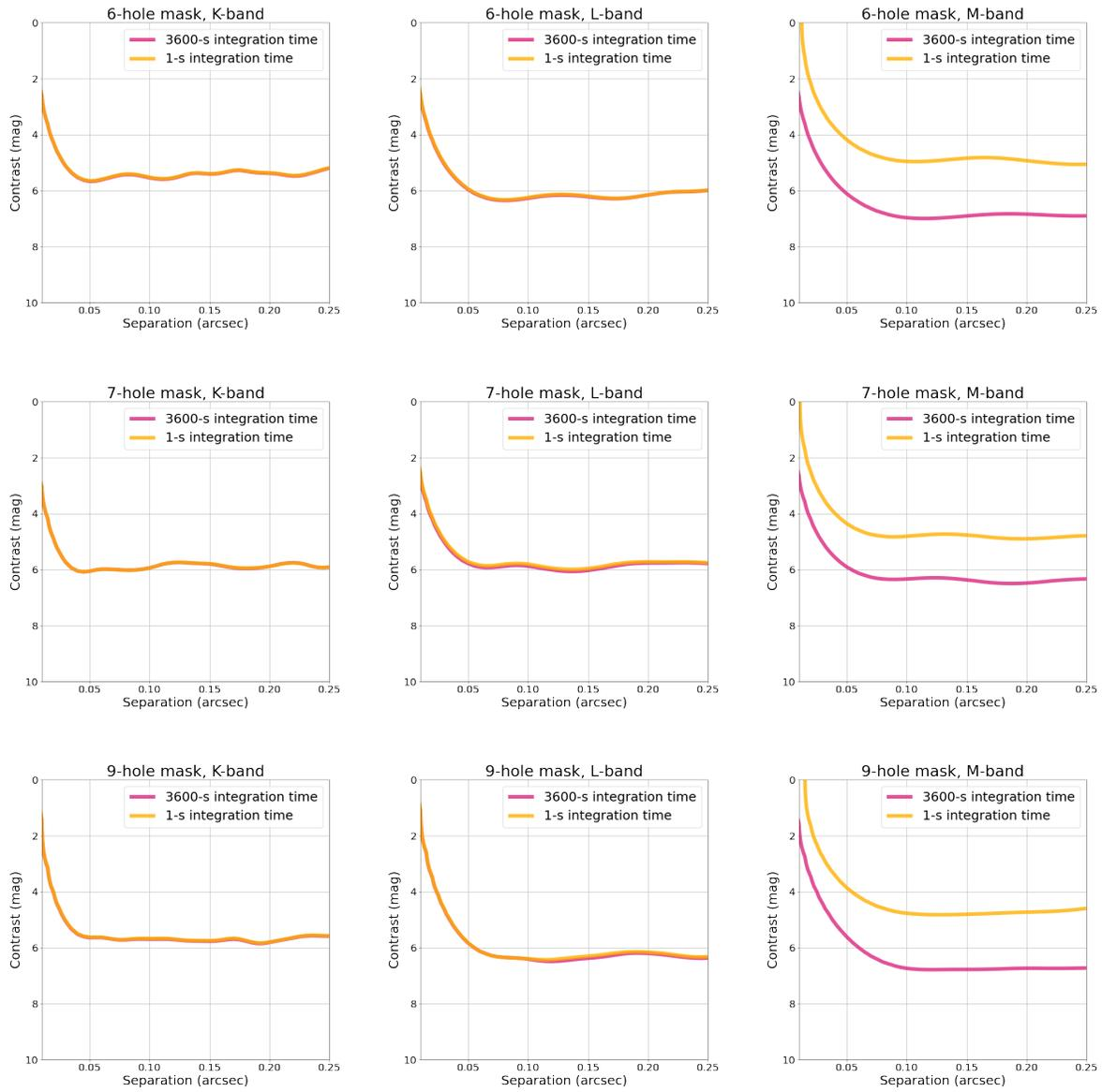
Figure 4.  $5 - \sigma$  contrast curves are shown for each mask and at each wavelength bin used:  $2.242\mu\text{m}$  (K-band),  $3.509\mu\text{m}$  (L-band), and  $5.019\mu\text{m}$  (M-band).
