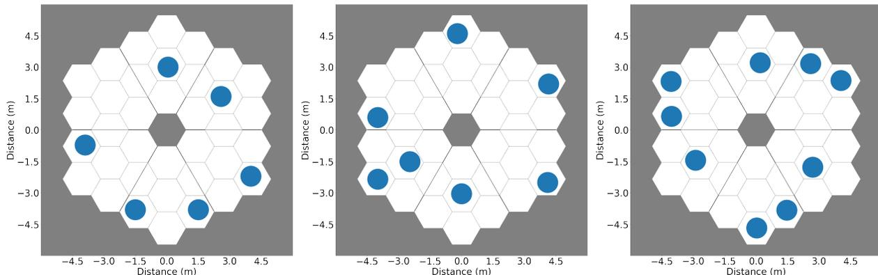
Figure 1. The three non-redundant sparse aperture mask designs used in this work. The mask holes are shown projected onto the 10m Keck primary mirror and measure 1m in diameter. From left to right: the 6-hole mask modified from the LBT design; a 7-hole design modified slightly from the VLT SPHERE mask; the 9-hole mask currently on Keck/NIRC2.
