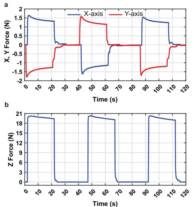
Fig. 4. Blocked force measurement results for single haptic voxel. The tactor produces approximately (a) 1.6 N in the  $x$  and  $y$  axes (parallel to the skin) and (b) 20 N in the  $z$  axis (normal to the skin). The corresponding actuators were activated and deactivated with periods of 20 sec. The soft tactor bends when actuated under the blocked condition and the material viscoelasticity causes force relaxation.
