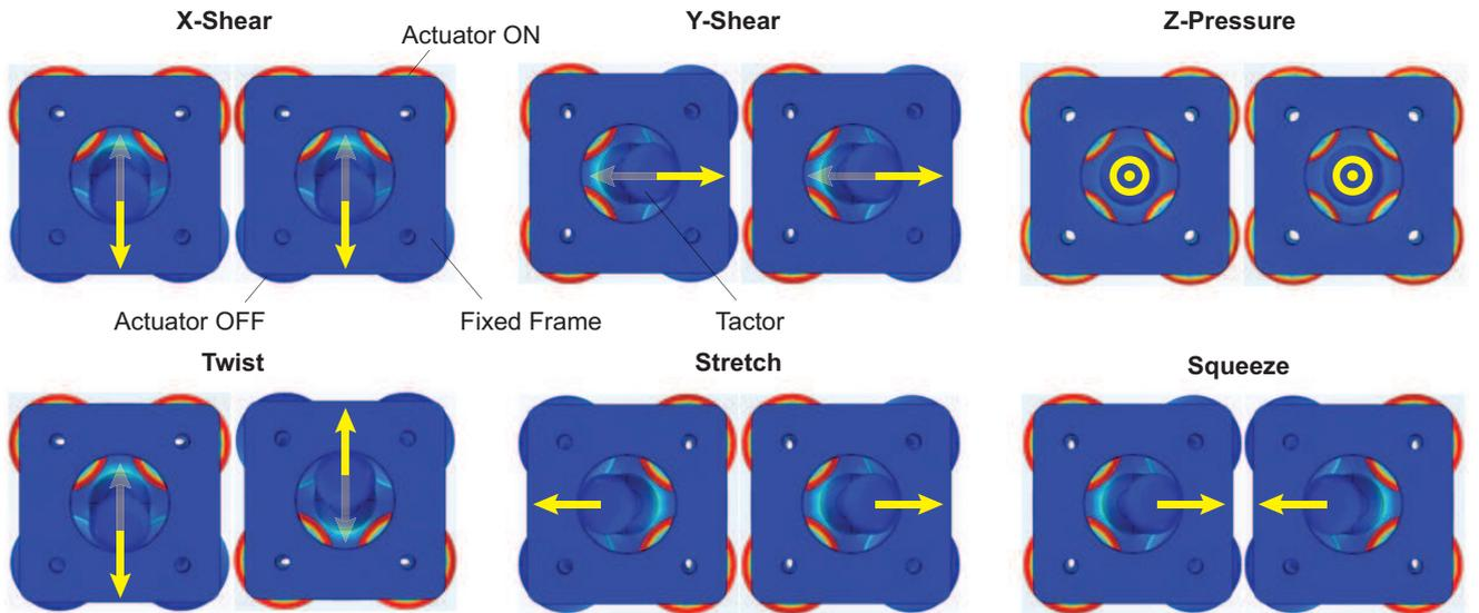
Fig. 3. Two hoxels can deliver diverse skin deformation stimuli: skin  $x$  and  $y$  shear,  $z$  pressure, twist, stretch, and squeeze. Although not illustrated here, the device can produce other arbitrary haptic stimuli owing to the tactors' freedom of motion.
