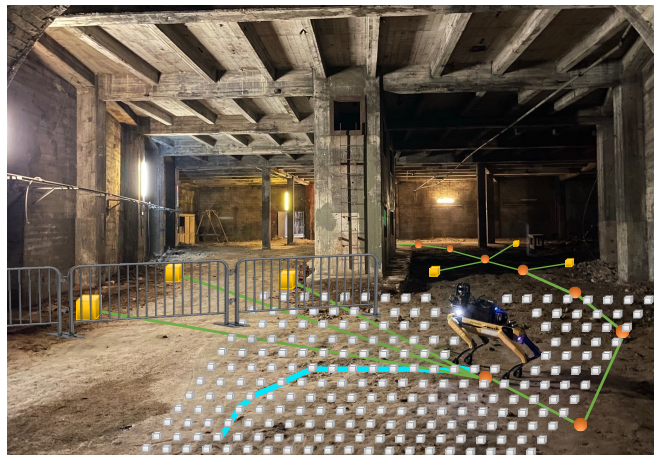
Fig. 1: An example of how meta-level decision making is used to balance the tradeoffs between local and global exploration. Global planning is conducted over the global IRM as shown by the orange spheres (breadcrumbs) connected by green edges. The yellow cubes represent global frontiers. Local planning is conducted over the local IRM (grid represented by gray cubes). In this case, the robot is currently following the global planner to reach the global frontiers shown by the yellow cubes on the left. However, the global frontiers are unreachable (behind the fence), requiring the robot to choose between following the local planner (cyan line) or relocating to a different global goal like those shown in the back right of the image.
