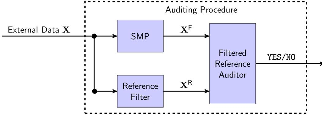
**Figure 2:** An illustration of the auditing procedure. The SMP and the uniformal filter get as an input the external data procedure, then output the filtered and the reference feeds, respectively. Both feeds are seen by the auditor, where the last outputs “YES” when the regulation is not violated, or “NO” otherwise.
