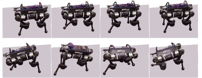
Fig. 13. Comparison between the nullspace and Schur-complement factorizations during a dynamic trotting gait with the ANYmal robot. The Schur-complement factorization is more expensive to compute, and our MPC cannot run at 50 Hz. These delays in the control loop produced instability in the trotting gait (bottom). Instead, the nullspace factorization allowed the MPC to run at 50 Hz and generated a stable trotting gait (top).
