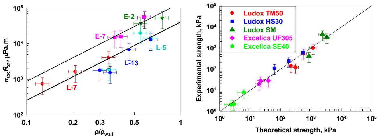
**Figure 7.** (A) Experimental data from Figure 5 plotted in the scale  $\ln(\sigma_{CR}R_p)$  vs  $\ln(\rho/\rho_{\text{wall}})$ . (B) Experimentally measured strength for all porous materials studied here, as a function of the calculated strength via eq.(11c) for the different silica particles used. The errors for the theoretically estimated strengths reflect the uncertainty in the particle size distribution. The
