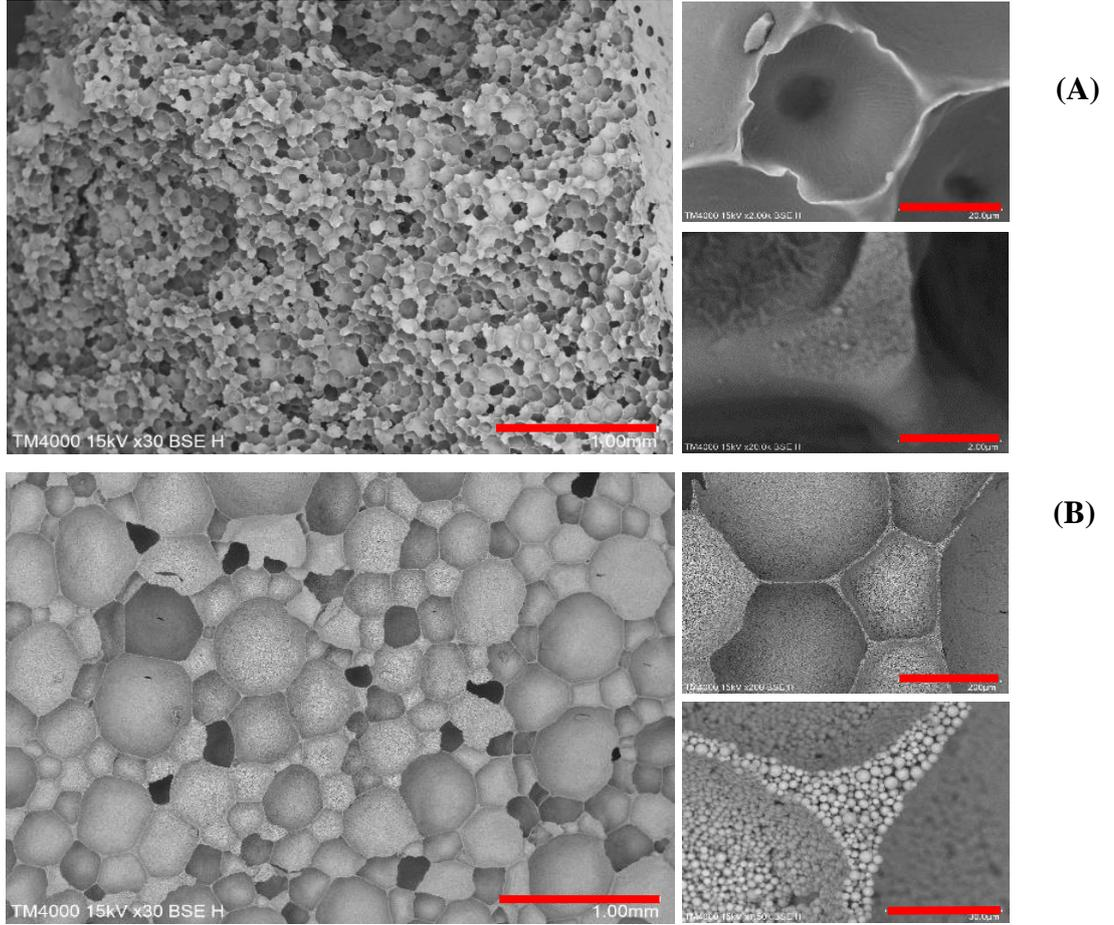
**Figure 6.** Microstructure of the porous materials with 76 vol% bubbles, prepared from (A) Ludox TM with  $R_{21} = 12.8$  nm precipitated silica particles and (B) Excelica 305 with  $R_{21} = 1.9$   $\mu\text{m}$  fused silica particles at different magnifications. Scales are 1000  $\mu\text{m}$ , 200  $\mu\text{m}$  and 30  $\mu\text{m}$ .
