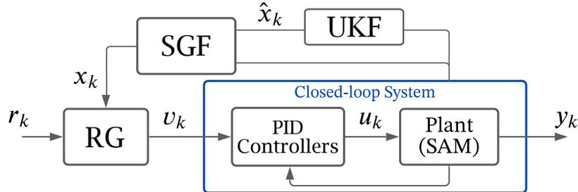
Figure 6: Block diagram visualizing the topology of the Reference Governor (RG) in conjunction with the Unscented Kalman Filter (UKF). A partial subset of the full state set,  $x_k$ , is predicted by the UKF algorithm,  $\hat{x}_k$ . Under the presence of noise, all outputs are denoised using the Savitzky-Golay filter (SGF).
