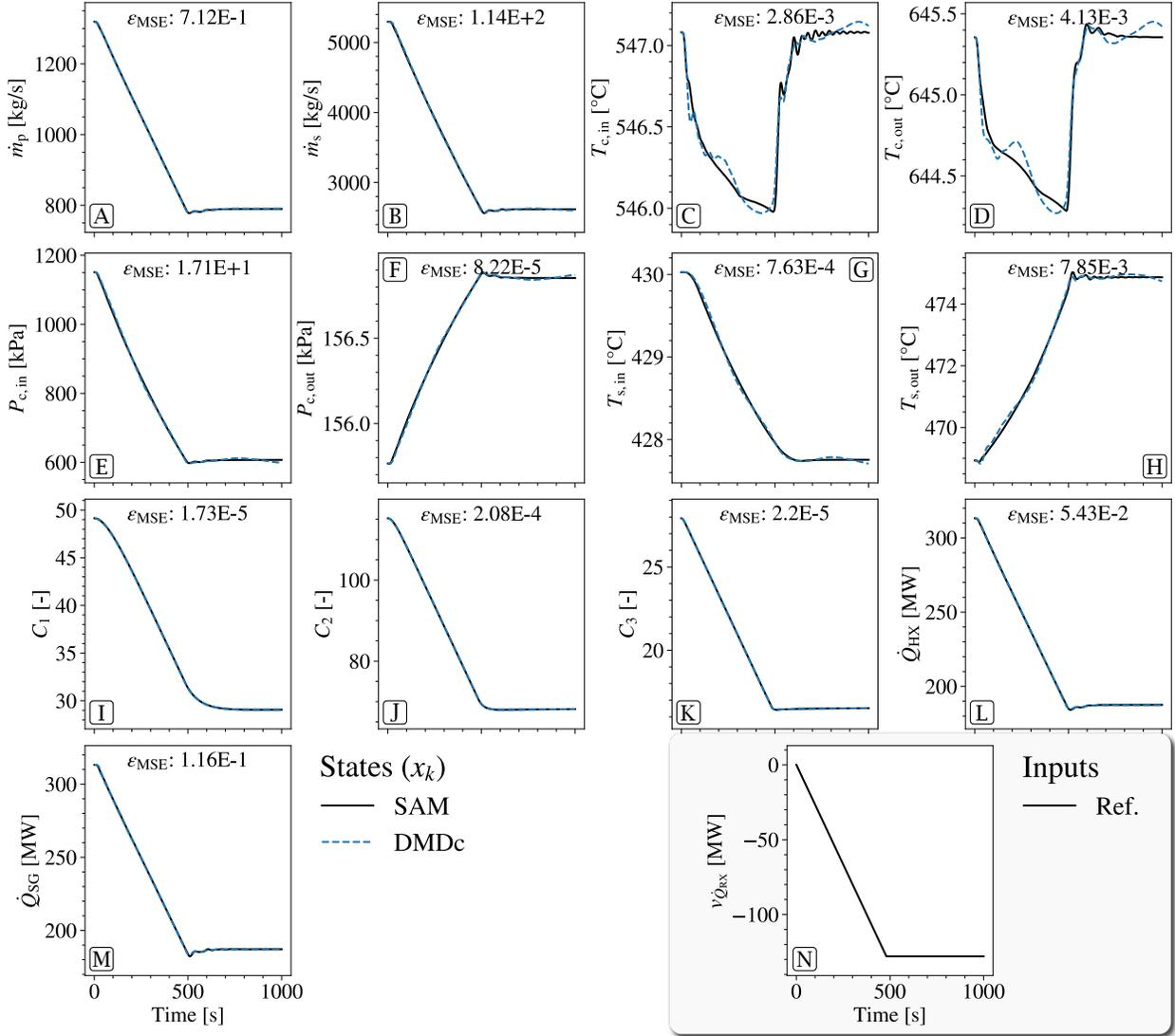
Figure 9: Assessment of the DMDc model accuracy during the 40 % load-follow transient. Gray box presents the reference input that is shared between all results in this section. Remaining plots display contrast of the propagation of states between the SAM model and the DMDc model. The mean square error,  $\epsilon_{MSE}$ , is inset in the subplot of each state.
