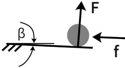
Fig.9 The force analysis diagrams when locking
