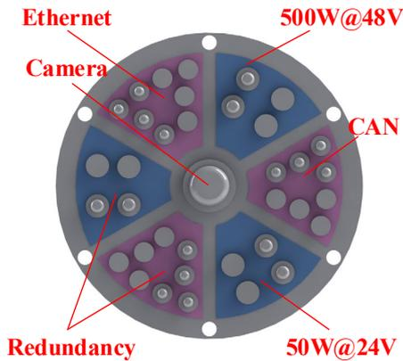
Fig.6 The power and data interface
