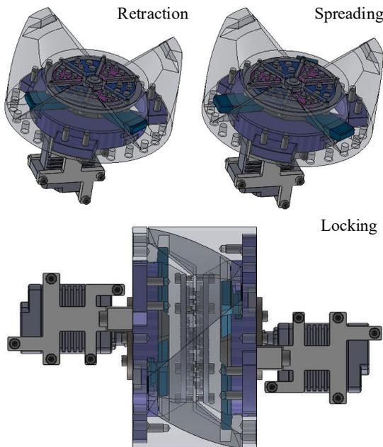
Fig.3 The CAD model of *PetLock*
