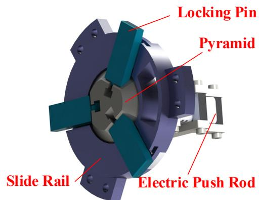
Fig.5 The Locking Mechanism
