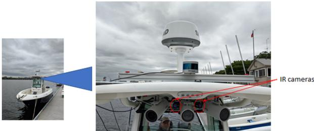
Figure 3. R/V Philos showing placement of LWIR cameras
