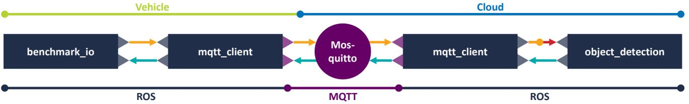
Fig. 3: Point clouds are published on the vehicle and transmitted to the cloud via MQTT, using two instances of `mqtt_client`. Before entering the object detection, the `VelodyneScan` point cloud messages are transformed to `PointCloud2` point cloud messages. Object lists are then computed from incoming point clouds and sent back to the vehicle. In- and out-timestamps are taken at each component, depicted as little triangles  $\triangleright/\triangleleft$ .
