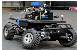
Fig. 1. One tenth scale CAV with camera, LIDAR, and Nvidia Jetson Nano for on-board processing.
