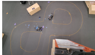
Fig. 3. Small ( s_l = 1.0m ) figure 8 loop with two CAVs and one CIS. Cardboard boxes around the track were placed for localization.
