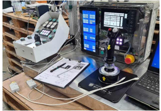
Fig. 5. Concept of the control center for teleoperation of road-marking machines
