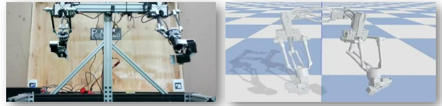
Fig. 1. Real-to-Sim. Here we show our experimental setup, where a manipulator robot is used to learn the residual error between the actual and simulated robot.
