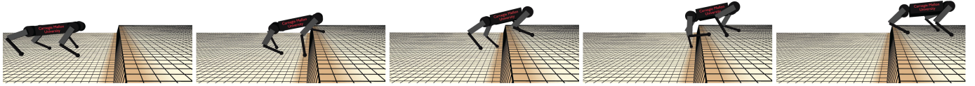
(a) The Step environment requires navigating kinematic constraints. Snapshots are shown of the trajectories under the Adaptive configuration. Non-steppable regions are indicated with darker shading.
