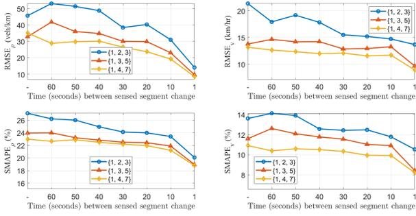
**Fig. 9.** RMSE $_{\rho}$  [top left], RMSE $_v$  [top right], SMAPE $_{\rho}$  [bottom left], and SMAPE $_v$  [bottom right] with different starting configurations of sensors and varying duration between changes in sensor positions using MHE. The symbol ‘-’ at the beginning of the x-axis represents the scenario with fixed sensor locations for the starting configurations in the legend.
