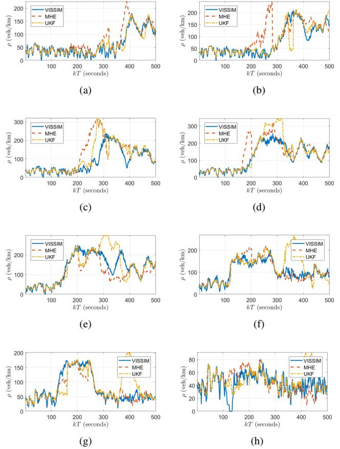
**Fig. 14.** Plots of simulated and estimated density trajectories on Segments 1 to 8 in the presence of 3 additional measured segments with changing positions using UKF and MHE. Figures from top to bottom on the left correspond to Segments 1, 3, 5, and 7, and on the right correspond to Segments 2, 4, 6, and 8.
