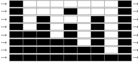
**Fig. 3.** Configurations for fixed sensor placement on the mainline segments. Black boxes depict segments with sensors and white boxes depict otherwise. Arrows indicate the direction of traffic. The ramp segments containing an additional 3 sensors are not presented in this figure. The top and bottom rows present the configuration with a total of 5 and 12 sensors in the system, respectively.
