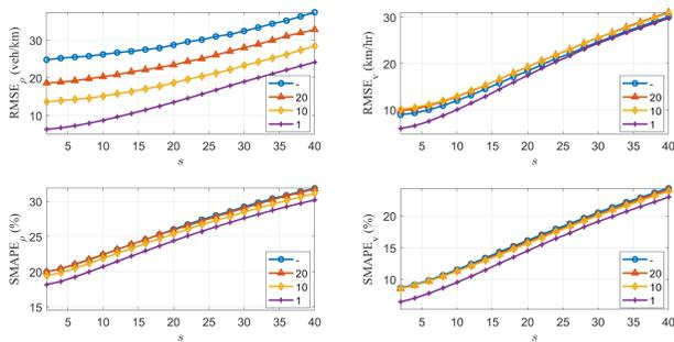
**Fig. 11.**  $RMSE_\rho$  [top left],  $RMSE_v$  [top right],  $SMAPE_\rho$  [bottom left], and  $SMAPE_v$  [bottom right] with changing  $s$  (standard deviation of added measurement noise) with 5 additional measured segments with changing positions using MHE.
