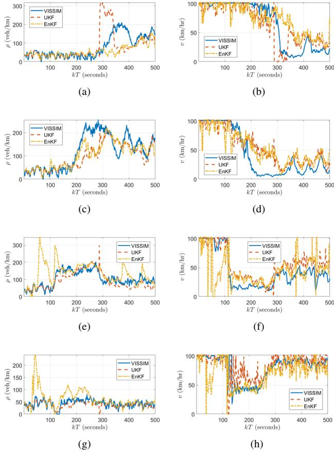
**Fig. 12.** Plots of simulated and estimated trajectories for densities [left] (a, c, e, g) and speeds [right] (b, d, f, h) in the presence of 4 additional fixed sensors using UKF and EnKF. Rows of figures correspond to the unmeasured Segments 2, 4, 6, and 8 respectively.
