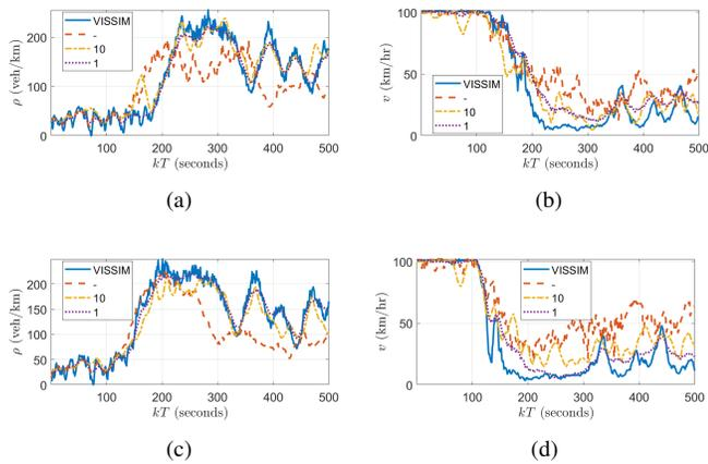
**Fig. 13.** Plots of simulated and estimated trajectories with smoothing for densities [left] (a, c) and speeds [right] (b, d) in the presence of 3 additional measured segments with changing positions and application of a smoothing filter. Rows of figures correspond to Segments 4 and 5 respectively.
