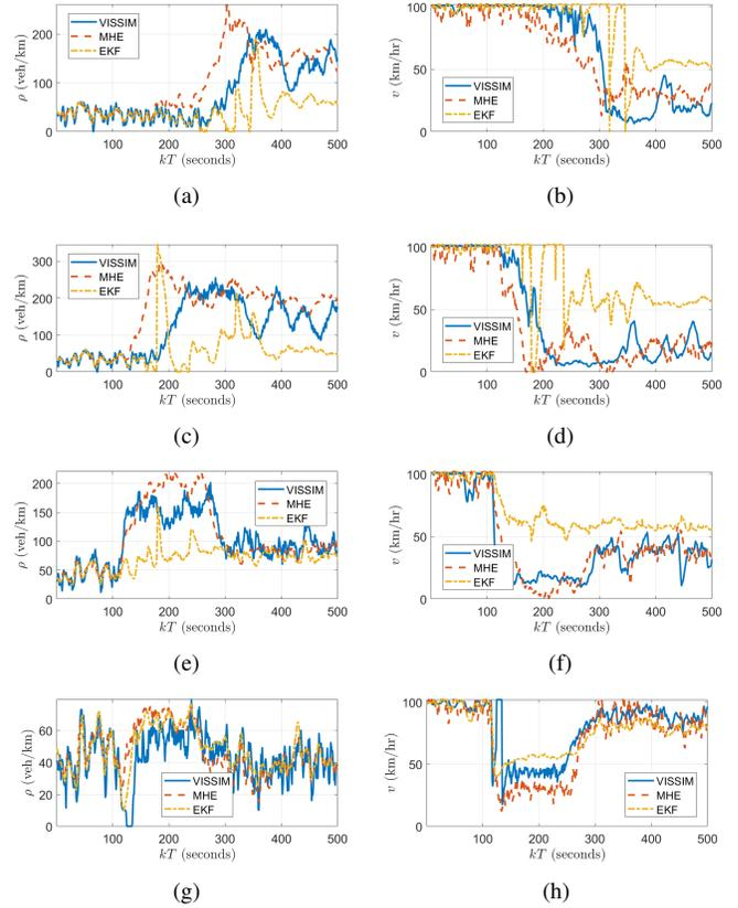
**Fig. 5.** Plots of simulated and estimated trajectories for densities [left] (a, c, e, g) and speeds [right] (b, d, f, h) in the presence of 4 additional fixed sensors. Rows of figures correspond to the unmeasured Segments 2, 4, 6, and 8 respectively.
