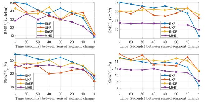
Fig. 7.  $RMSE_\rho$  [top left],  $RMSE_v$  [top right],  $SAMPE_\rho$  [bottom left],  $SAMPE_v$  [bottom right] with different duration between changes in sensor positions. The symbol ‘-’ at the beginning of the x-axis represents the scenario with fixed sensor locations throughout the simulation.
