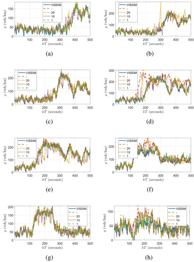
**Fig. 15.** Plots of simulated and estimated density trajectories on Segments 1 to 8 in the presence of 5 additional measured segments with changing positions and  $s = 22$  with MHE. Figures from top to bottom on the left correspond to Segments 1, 3, 5, and 7, and on the right correspond to Segments 2, 4, 6, and 8.
