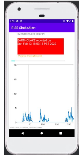
Figure 3: Moderate shaking detected by device which are reported to the server. This is a screenshot after the shaking report was sent to the server and the earthquake warning received back from the server. An audible alarm is also triggered on every device.
