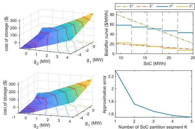
Fig. 2: Top left: nonconvex true storage cost in 2-interval. Top right: true SoC-dependent marginal cost and optimal EDCR approximation bids ( $K = 5$ ). Bottom left: optimal EDCR approximation cost in 2-interval. Bottom right: EDCR approximation error.
