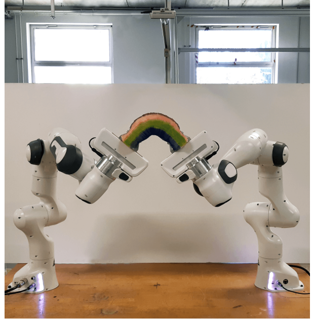
Fig. 1. Our experimental setup with two Franka robots manipulating a foam octagonal cylinder. An overhead 3D camera provides the input for our approach.
