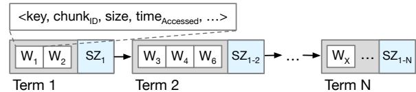
Figure 6: An example insertion log. W_1 denotes the first PUT record stored under Term 1.
