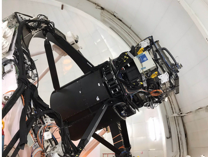
Figure 1. The assembled top end of WEAVE on the William Herschel Telescope in La Palma, Spain. This photo was taken on the 25 th of May 2022.
