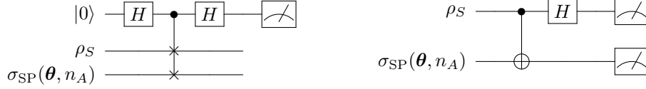
FIG. 8. Two circuits to evaluate \text{Tr}[\rho_S \cdot \sigma_{\text{SP}}(\boldsymbol{\theta}, n_A)] or \text{Tr}[\sigma_{\text{SP}}(\boldsymbol{\theta}, n_A)^2] by choosing \rho_S = \sigma_{\text{SP}}(\boldsymbol{\theta}, n_A) . (Left) A version of the SWAP test as first discussed in Ref. [45]. For completeness, we demonstrate that this circuit works as intended from Eq. (B3) to Eq. (B8) since Ref. [45] is not explicit for our context. This requires an ancilla and a controlled swap (aka Fredkin) gate. As the proof will show, this circuit can be straightforwardly generalized to n qubit states by performing an 2n qubit SWAP rather than a two qubit SWAP. (Right) A destructive variant of the SWAP test discovered in the context of optical systems and the Hong-Ou-Mandel effect in Ref. [46]. This removes the need for ancilla and a complicated Fredkin gate but destroys the prepared states in the process in what is known as a Bell measurement . Much of Ref. [46] is dedicated to showing the right circuit is equivalent to the left circuit, so we do not re-derive the entire result here. Instead, we comment on how to connect the measurements of the circuit to the desired quantity in Eq. (B10). We then discuss how to generalize this procedure to n qubit mixed states in Eq. (B11).
