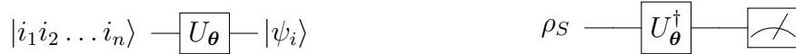
FIG. 9. We summarize the circuits used to evaluate the cost function for the CCPS ansatz. (Left) A generic way to prepare a randomly sampled eigenvector of the CCPS state. Here, the state |i_1 i_2 \dots i_n\rangle is a short-hand for an n qubit computational basis state, so each i_j is either 0 or 1. Given the randomly sampled bitstring, we can prepare the desired state with single qubit X gates, and then we apply the same unitary U_\theta regardless of the randomly sampled input. (Right) Here, we provide a circuit to sample the distribution q_\theta(i) defined in (B14). We simply prepare \rho_S , apply U_\theta^\dagger , and measure each qubit separately in the computational basis. By (B14) and the fact that p_\phi(i) is stored classically, we can therefore compute the desired cross term using a classical SWAP test as described in the main text around (24).
