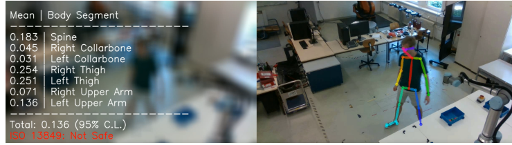
Fig. 5. Our method allows to estimate the uncertainties on user-selected joint pairs online. During run-time, our method provides uncertainty values and an evaluation on an arbitrary safety limit (e.g., ISO 13849).
