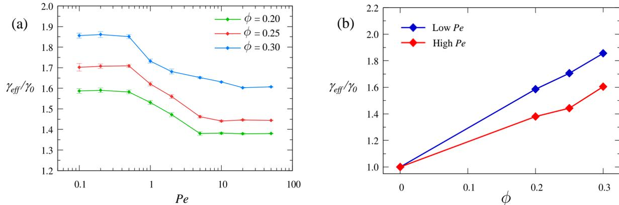
FIG. 2. (a) Dependence of the friction coefficient with  $Pe$  in I phases of HBPs with  $L^* = 12$  and  $W^* = 3.46$  at  $\phi = 0.20, 0.25$  and  $0.30$ . (b) Variation of  $\gamma_{\text{eff}}/\gamma_0$  at high and low  $Pe$  at different  $\phi$ . The lines are guides for the eye.
