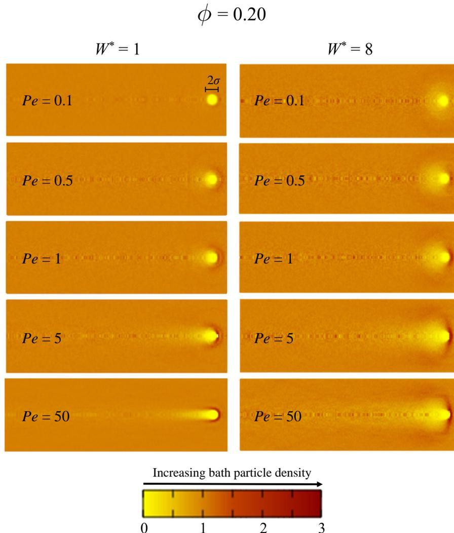
FIG. 5. Density maps of HBPs with  $\phi = 0.20$  at  $W^* = 1$  (left) and  $W^* = 8$  (right) and at the  $Pe$  numbers indicated in each frame. The colour palette is shown on at the bottom of the figure and refers to the ratio between the local density and the bath density. Yellow regions indicate low bath particle density, while the dark red regions indicate high bath particle density.
