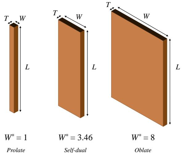
FIG. 1. Model HBPs studied in this work. Length, width and thickness are respectively labelled as  $L = 12T$ ,  $W$  and  $T$ , with  $T$  the system unit length. The reduced width,  $W^* \equiv W/T$ , assumes three different values to reproduce prolate, self-dual and oblate geometries.
