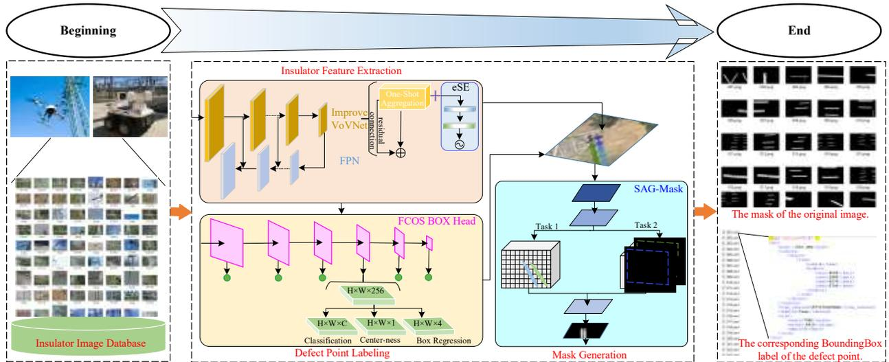
**Figure 1** The overall framework of the intelligent detection method for insulator defects
