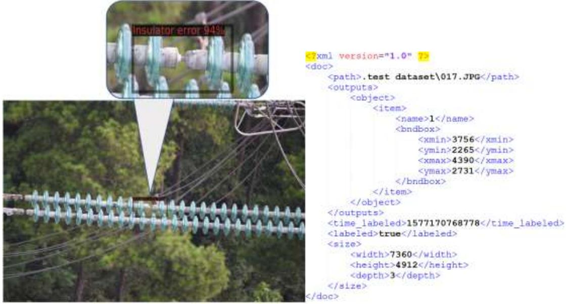
**Figure 3** The insulator defect point detection and positioning.
