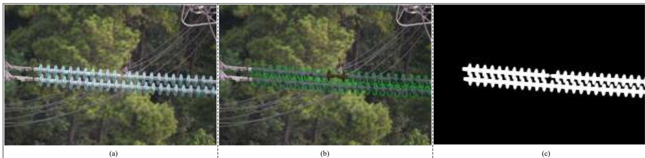
**Figure 2** The insulator mask generation process: (a) Original image of insulator beading. (b) Annotated drawing of the insulator. (c) Insulator mask extraction.
