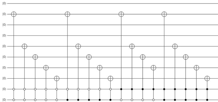
Figure 1: Quantum circuit for the GQIR representation of a  $2 \times 2$  gray scale image
