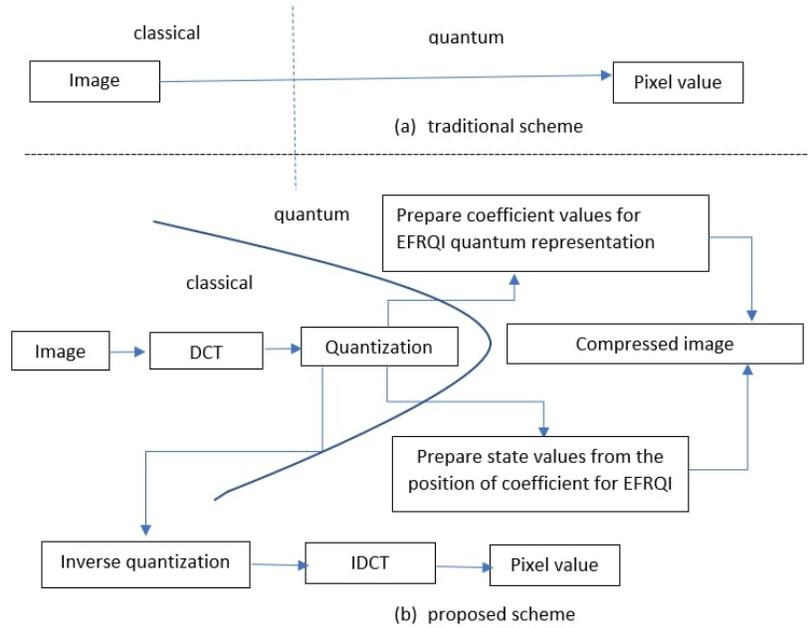
Figure 3: Basic idea of proposed scheme and difference with traditional scheme.
