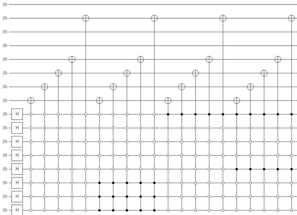
Figure 2: An  $16 \times 16$  GQIR-DCT quantum image and its quantum state
