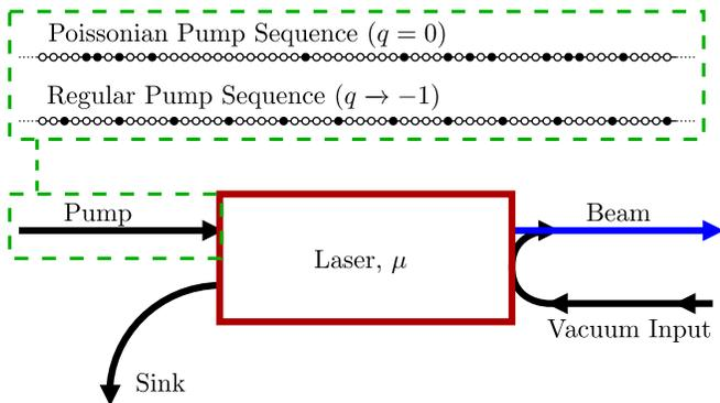
FIG. 1. Basic schematic of a laser showing the key components of the two families of models discussed in the text. Top green box depicts different statistics for the pump, applicable to the  $q$ -family, while the  $\lambda$ -family is constrained to have Poissonian pumping statistics.
