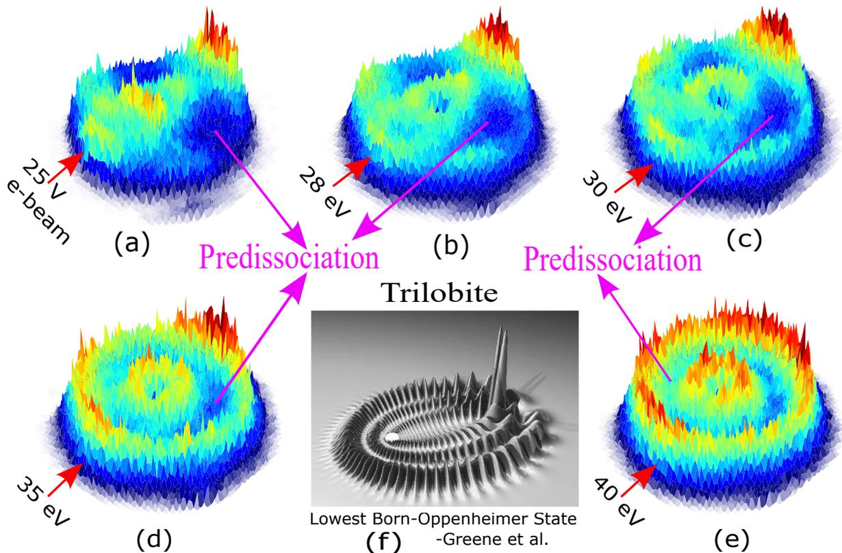
FIG. 1. The surface plots (a,b,c,d, and e) depict the wedge slice images of  $O^-/CO$  extracted from electron-induced IPD dynamics for CO using state-of-the-art momentum imaging apparatus at incident electron energies 25, 28, 30, 35 & 40 eV, respectively. (f) The lowest Born-Oppenheimer state as reported by Greene *et al.* [1]. The red arrows indicate the induced electron beam direction labelled with the energy values.
