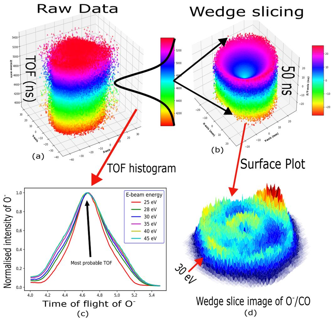
FIG. 6. (a) MCPs and Hex-anode detected raw data, (b) Scatter plot of the wedge sliced data, (c) Time of flight histogram of the detected  $O^-$  fragments, and (d) the surface plot of the wedge-shaped data.
