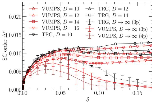
FIG. 13. Comparison of the SC order for  $d+id$ -wave uniform states between two methods, VUMPS and TRG. For  $D \rightarrow \infty$ , the line labeled by “3p” is extrapolated using three data points with  $D=10, 12, 14$ , and the line labeled “4p” is extrapolated using four data points with  $D=10, 12, 14, 16$ . Generally, the SC order from TRG calculation is larger than the one from VUMPS calculation for each  $D$  and the extrapolation.
