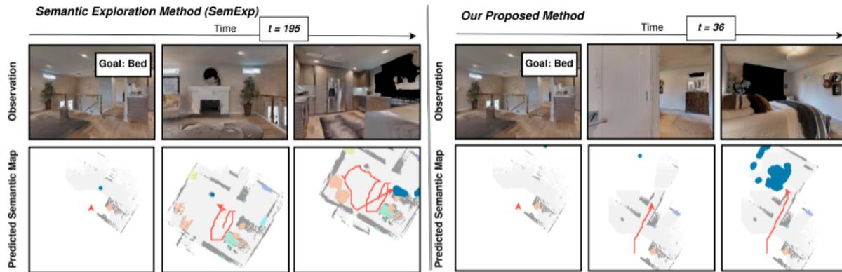
Fig. 3: **Qualitative Comparison with SemExp baseline:** Snapshots from a paired trial comparing our framework (right) with the SemExp baseline [2] (left) in a particular scene. With each method, the robot starts at the same location with the same target object class ‘bed’. Our framework results in an instance of the target object class being found much faster.
