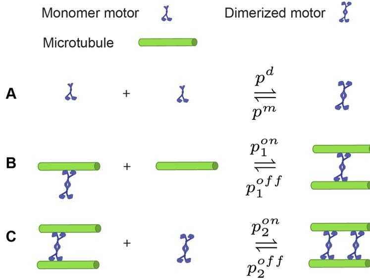
FIG. S2: **Illustrations of chemical reactions in the model.** **A**, Reversible dimerization of motors. **B**, Reversible crosslinking of a freely-moving microtubule  $i$  and another microtubule  $j$ . The latter can be either free or pre-crosslinked. **C**, Reversible binding of a dimer motor on two pre-crosslinked microtubules.
