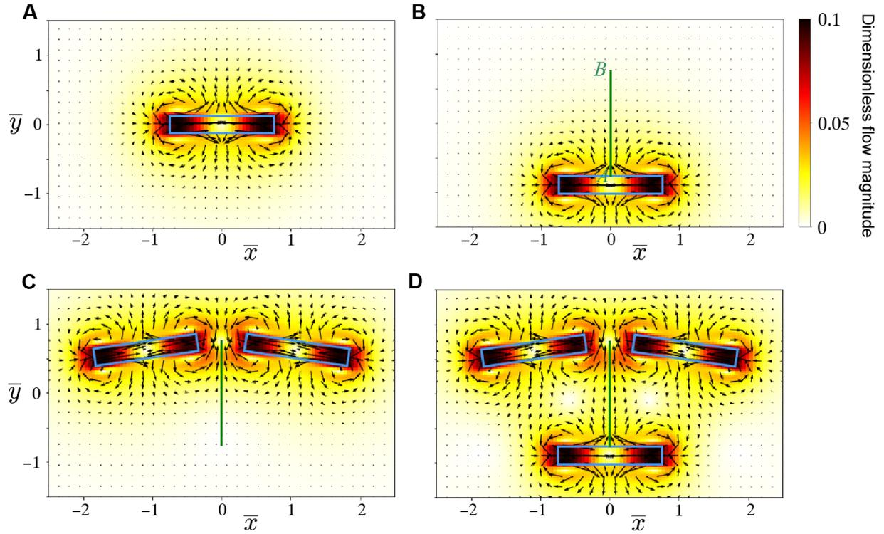
FIG. S4: **A**, Simulated single-bar flow field. Optimal solutions for particle transport using **B**,  $n = 1$ , **C**,  $n = 2$  and **D**,  $n = 3$  light bars, and their corresponding flow fields. The objective is to move a particle along the line segment AB (green). The outlines of light bars are plotted in blue.
