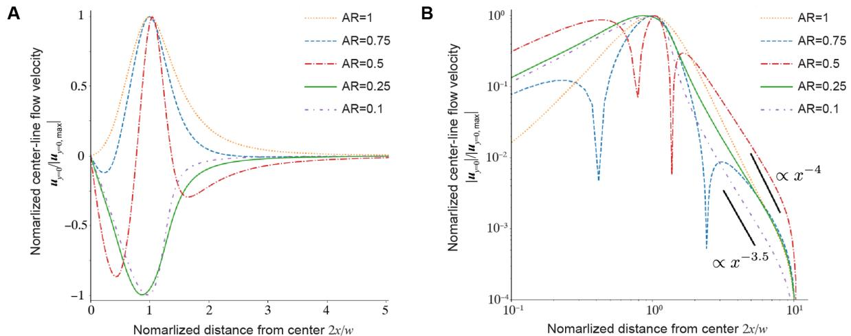
FIG. S3: **A**. Simulated center-line flows induced by single bars with different aspect ratios (AR). Positive (negative) values represent the flow is directed away from (into) the light bar. **B**. Absolute values of data in **A** in a log-log plot.
