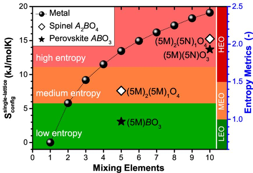
Figure 2. Visualization of difference in entropy evaluation by single lattice model used for metals and entropy metrics used for complex oxides<sup>33</sup>.
