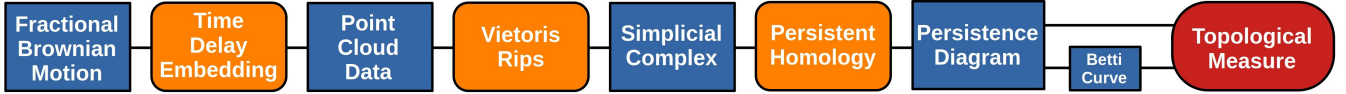
FIG. 4. The proposed pipeline in this paper: A synthetic fractional Brownian motion (fBm) time series is converted to a point cloud data (PCD) by the time-delay embedding (TDE) method. The evolution of homology groups of simplicial complex mapped from the constructed point cloud data by the Vietoris-Rips (VR) method is calculated by the persistent homology (PH) technique and summarized as persistence pairs (PPs) in persistence diagrams (PDs). Finally, topological measures based on the persistence diagrams and Betti curves are computed.
