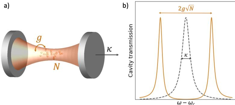
**Fig. 1** a) An illustration of an open Tavis-Cummings system consisting of an optical cavity of the loss rate  $\kappa$  with  $N$  atoms each coupled at the interaction rate  $g$ . b) The transmission spectrum of an empty cavity (dashed gray line) featuring a lorentzian profile with linewidth  $\kappa$  and a cavity resonantly coupled to  $N$  atoms (solid orange line) featuring two polariton peaks separated by  $2g\sqrt{N}$ .
