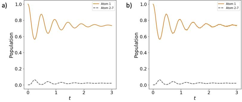
**Fig. 3** The evolution of the singly excited open quantum system Tavis-Cummings model of  $N = 7$ ,  $g = \kappa = 5$  calculated using a) quantum master equation in QuTiP software [37, 38] and b) Q-MARINA algorithm in QASM simulator with 40,000 shots per data point.
