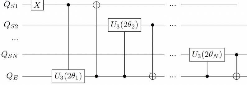
**Fig. 2** Q-MARINA algorithm that maps an open quantum system of  $N$  two-level atoms in a lossy cavity to a quantum circuit with  $N + 1$  qubits and  $2N$  entangling gates that encode the interaction of atoms ( $Q_{S_n}$ ) with the cavity and environment ( $Q_E$ ).
