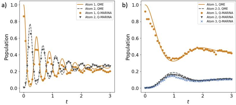
**Fig. 4** Q-MARINA simulation of the singly excited open TC system for evolving upon excitation of the Atom 1, executed on a) `ibmq_qui` to quantum computer with 10,000 shots per point for  $N = 2$ ,  $g = 10$ ,  $\kappa = 5$ , and b) `ibmq_oslo` quantum computer with 10,000 shots per point for  $N = 3$ ,  $g = 2$ ,  $\kappa = 5$ . The exact QME solution is plotted for comparison.
