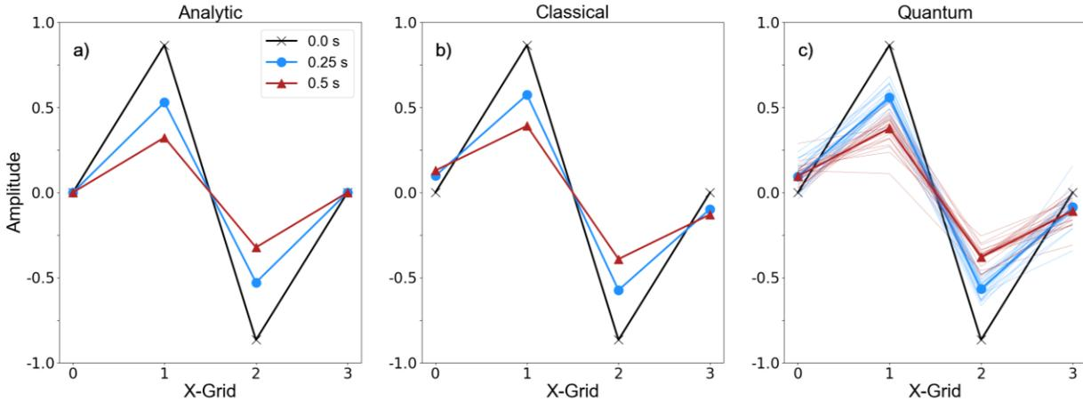
**Fig. 4** Solutions to the advection-diffusion equation at three time steps for the a) analytic solution, b) classical solution of the linear system of equations discussed in the text, c) same as (b) except for the quantum solutions of the 24 different runs on IBM’s quantum hardware (thin lines) and average of the 24 runs (thick lines). For all plots the initial condition is shown in black, 0.25 s time step in blue, and 0.5 s time step in red.
