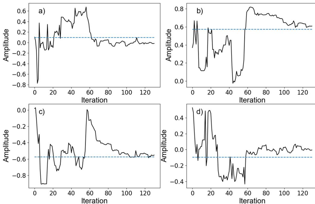
**Supplemental Figure 1** Convergence of the solution in black at the 0.25 s time step as a function of iteration for a) grid point 1, b) grid point 2, c) grid point 3, and d) grid point 4. The dashed blue line is the classical solution for which the quantum solution is expected to converge onto. This particular run was performed on the IBM's Cairo machine.
