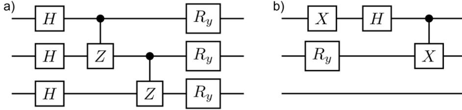
**Fig. 2** a) A unit of the ansatz that is repeated in the full quantum circuit depending on the specified circuit depth. H is the Hadamard gate, Z is the Pauli Z-gate, and  $R_y$  is the rotation gate about the y-axis for angle  $\theta$  discussed in text. b) The quantum circuit used to prepare the b-vector. X is the Pauli X-gate, and the angle  $\phi$  is used to rotate  $R_y$ .
