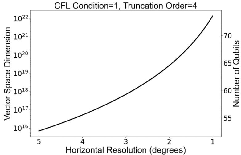
**Fig. 1** The vector space dimension required to solve the advection-diffusion equation using the methods discussed in this paper as a function of the horizontal resolution of a two-dimensional 10-day global forecasting model. The right y-axis shows the number of qubits required to process a corresponding Hilbert space of equal or greater dimension on a quantum computer.
