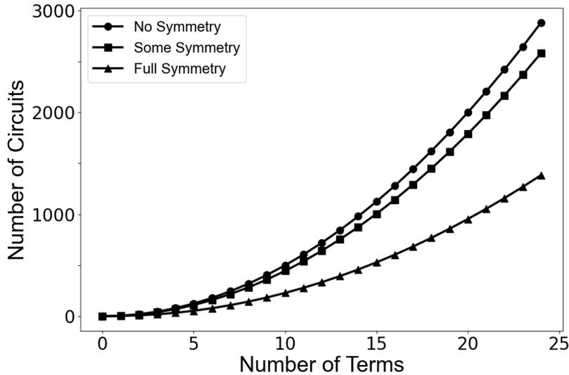
**Fig. 5** The number of circuits required as a function of the number of terms in the Pauli decomposition of the matrix A. Three cases are shown with various amounts of circuit symmetry used to reduce the total number of circuits (see text for discussion).
