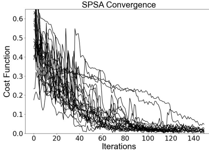
**Fig. 3** The local cost function as a function of the iteration using the SPSA optimization method for the 24 real QC runs.
