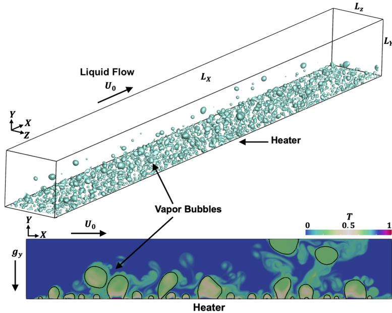
Figure 4: Example of a flow boiling simulation with Flash-X. Liquid coolant flows over a heater surface with a mean velocity  $U_0$ , leading to phase-change and formation of vapor bubbles. The bubble dynamics introduce turbulence which enhances heat transfer between the heater surface and coolant, shown by temperature ( $T$ ) contours
