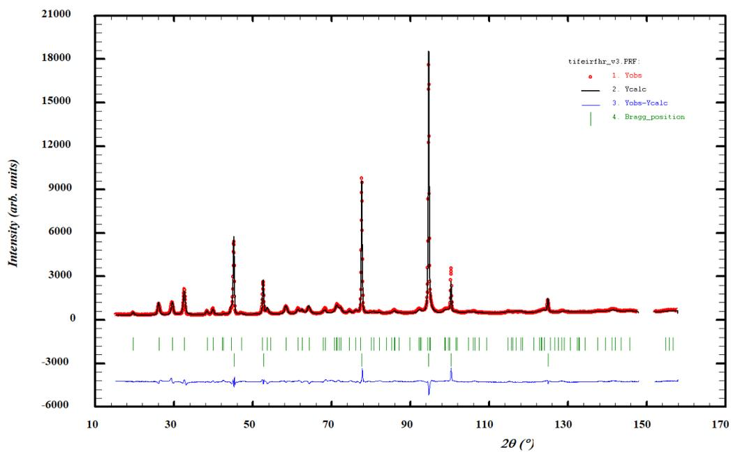
**Figure S3** – Neutron diffraction pattern and Rietveld refinement of the  $\gamma$  phase of sample B (scan number 25,  $\text{TiFe}_{0.85}\text{Mn}_{0.05}$ ) recorded at ILL beamline D2B at RT.
