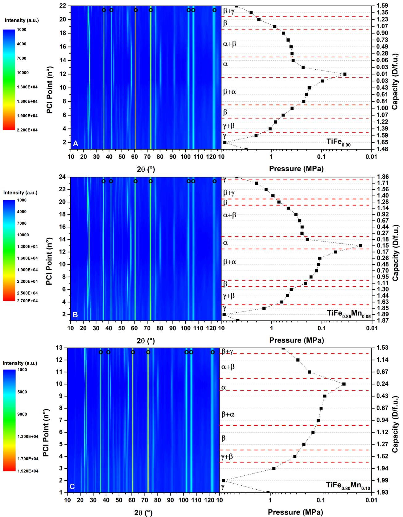
**Figure 2** – *In-situ* neutron diffraction patterns (counter plot) and PCI curve at RT during deuterium absorption/desorption at ILL between 0.02 and 9 MPa for sample A (top), B (middle) and C (bottom) at RT. Diffraction lines from the stainless-steel sample holder are marked by a circle (o).
