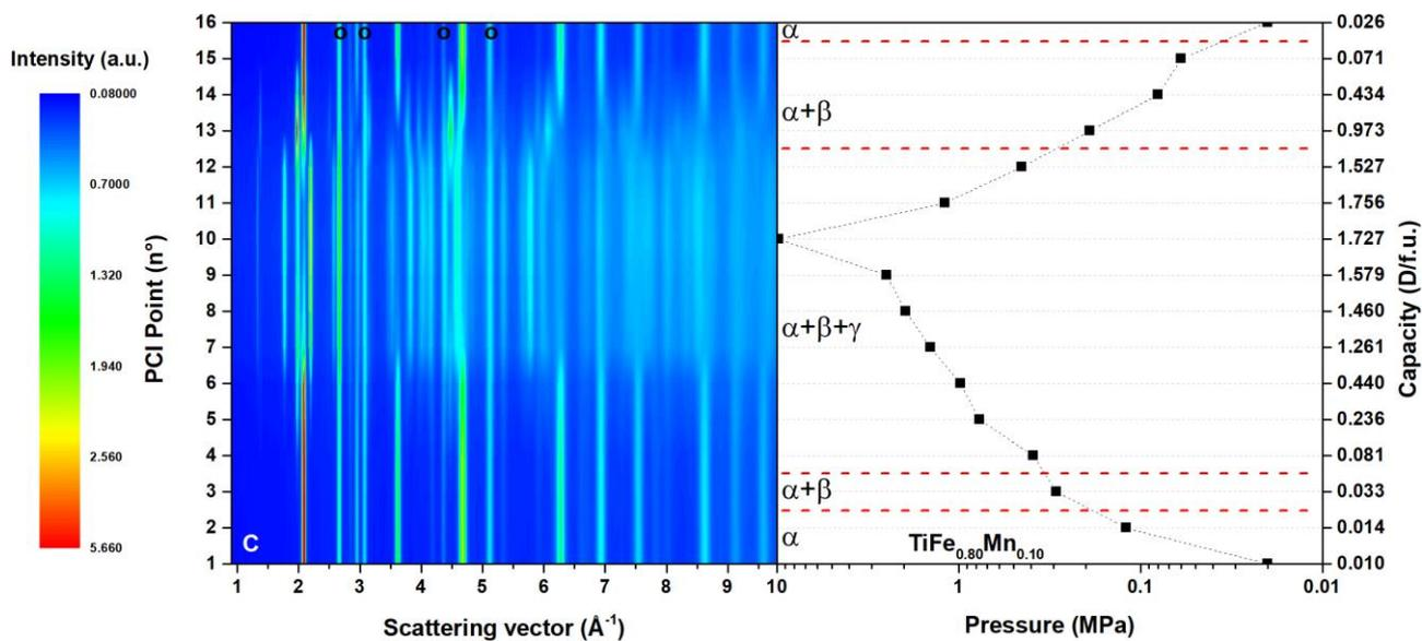
**Figure 3** – *In-situ* neutron diffraction patterns (counter plot) and PCI curve during deuterium absorption/desorption at ISIS between 0.02 and 9.8 MPa for sample C at RT. Diffraction lines from the aluminium sample holder are marked by a circle (o).
