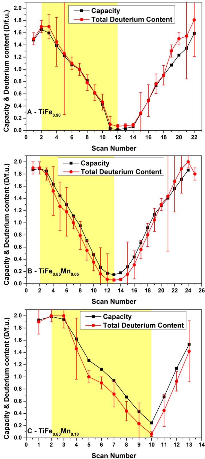
**Figure S1** – PCI determined capacity at ILL and total deuterium content determined by Rietveld refinement as a function of scan number for sample A, B, and C. Yellow area is evidencing desorption determinations, while white area refers to absorption. Scan numbers correspond to PCI points reported in the manuscript.
